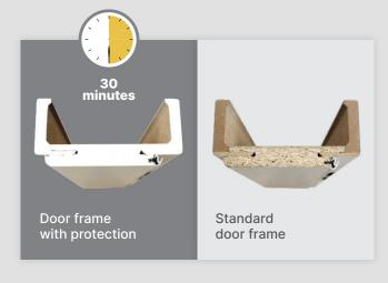
The adjustable door frame with innovative bottom edge protection, subjected to a 30-minute immersion in water, showed significantly higher resistance to absorption compared to the version without protection.
